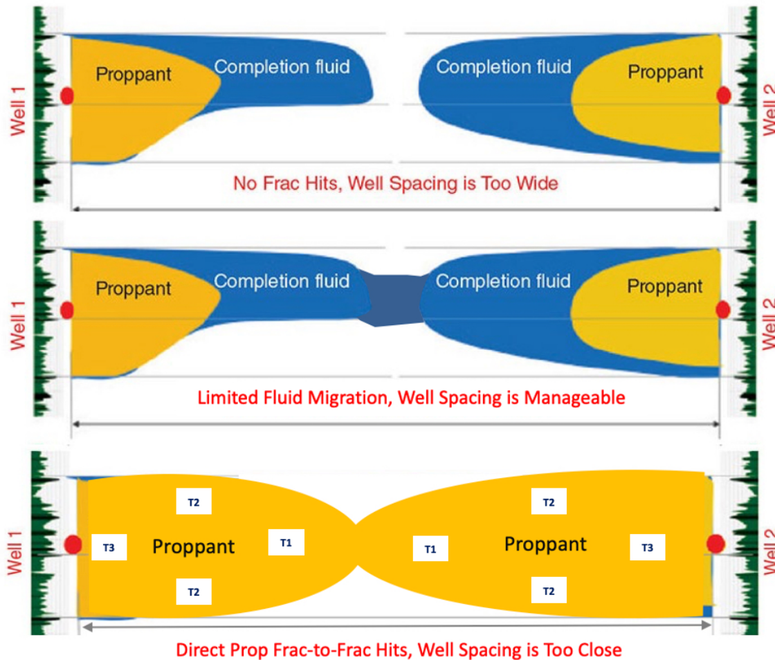
Figure 2: The various types of frac hits and their respective impact on production and EUR (Shokanov et al. 2021).
