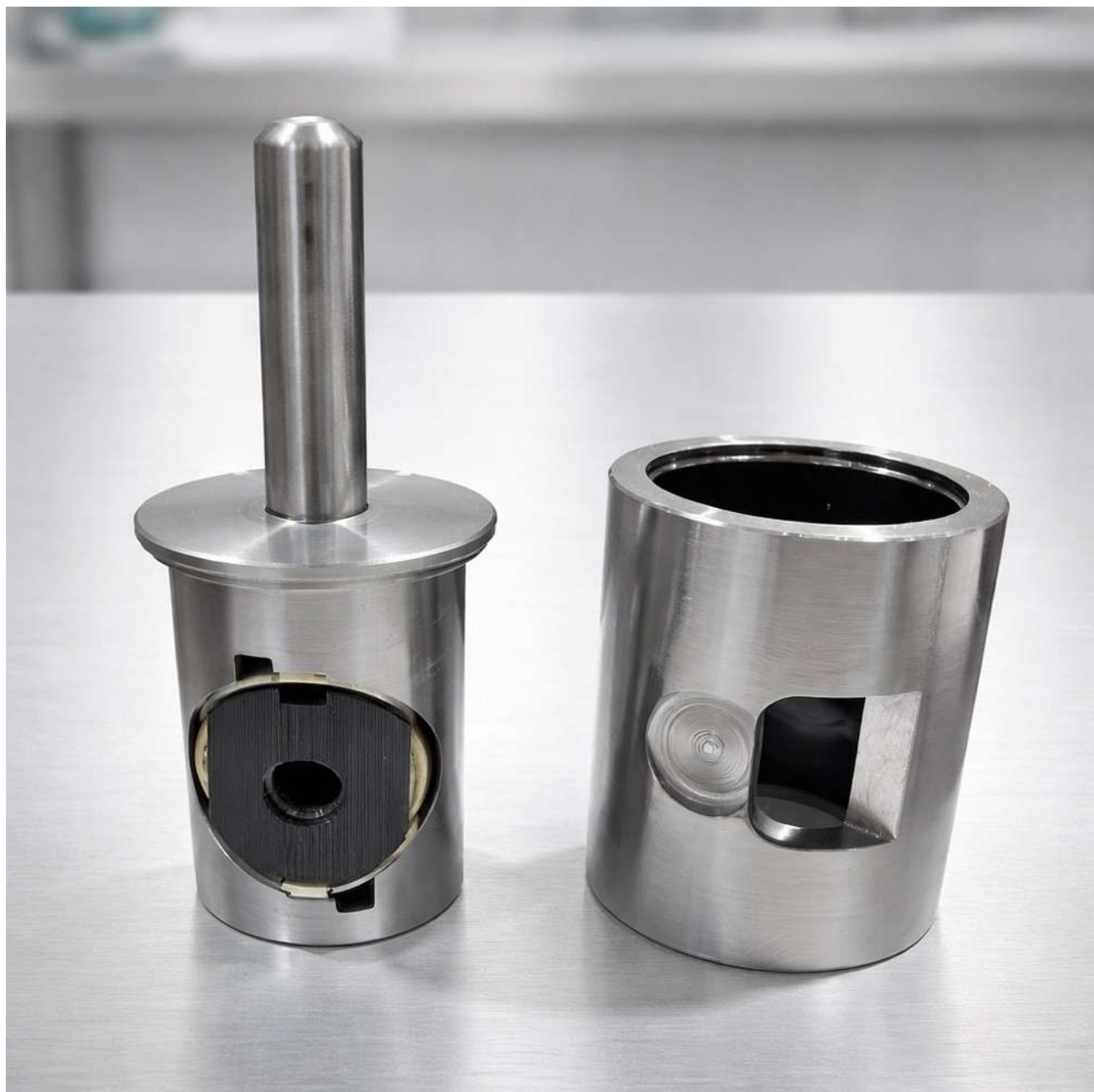
Fig. 2. Custom (non-OEM) insert cartridge installed (left) and charge holder body (right).
