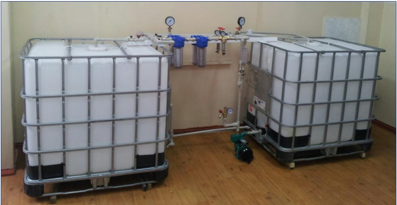
Figure 3: Testing unit for flow profile and recovery performance analysis
