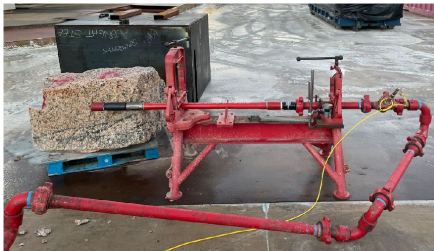
Fig. 9—Abrasive Jetting Test Setup with a Granite Boulder.
