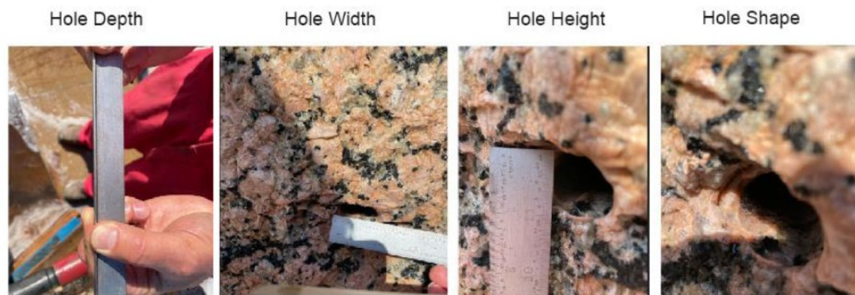
Fig. 10 Abrasive Jetting Result from a 1.1 bpm Test.
